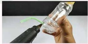
**Step-4**: Make a hole at the bottom of a plastic bottle. After that, attach a straw in the hole by using a glue gun and keep the bottle in the box.
